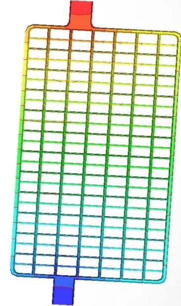
The structural design of positive plate has been modified and adapted in thickness in order to achieve lower a lower Pavlov  $\gamma$  factor, so that the cyclic performance and charging acceptance can be improved
