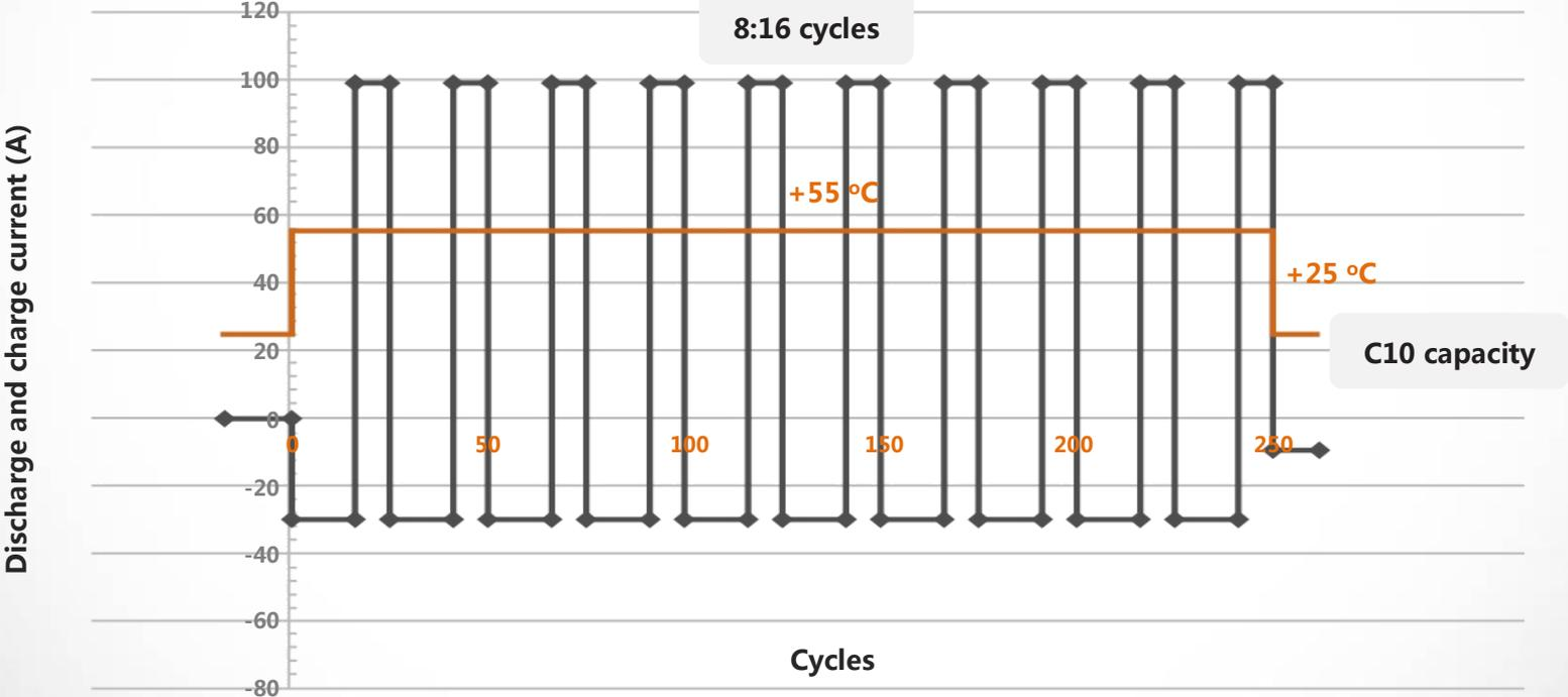
Test condition: under 55 degrees, 80% DOD, and recharge time of 8 hours
