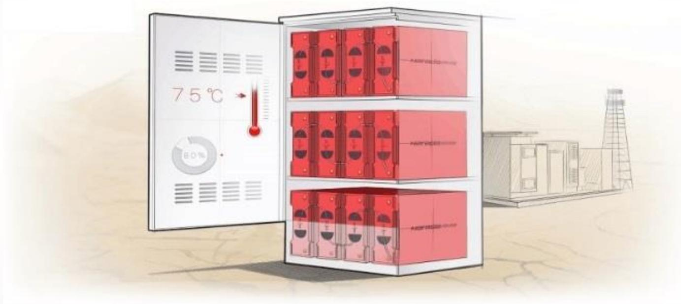
Most those appliances applied in telecom sites could be operated under higher temperature, such as: wireless units (5°C ~ 55°C); power supply (-5°C ~ 40°C); A/C equipment (5°C ~ 55°C). However for batteries, the suggested temperature should be 25°C, otherwise battery life will be reduced by 50% per each additional increased **10°C**
