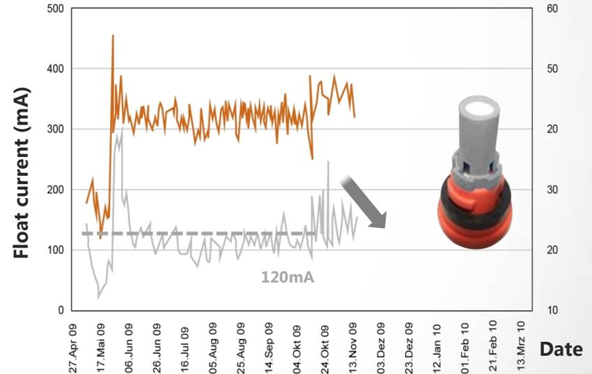
Under elevated operating temperature (above 40°C), the float current and temperature of 12V100Ah conventional monobloc is much higher than the one that is equipped with catalyst valve in each cell
