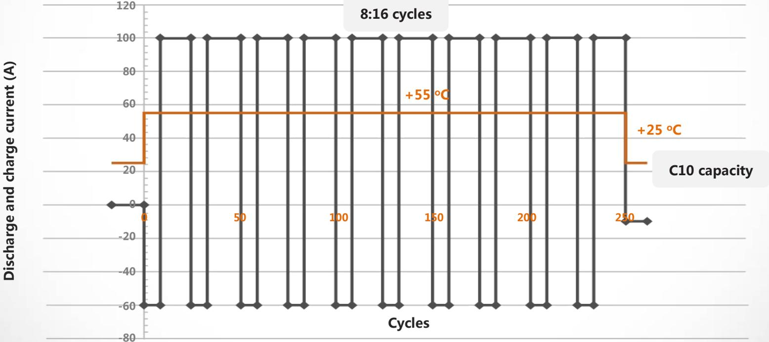
Test condition: under 55 degrees, 80% DOD, and recharge time of 16 hours
