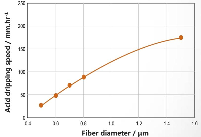
The diameter of fiberglass on separator is an important factor: bigger diameter is good for keeping wet elasticity, while smaller one is good for acid dripping. We found most rational proportion by many tests
